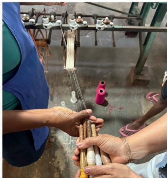
Since my fabric yarn was twisted together with different colours of yarn they rewind a new bobbin with previously winded bobbins while twisting them
