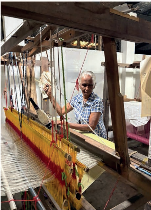
Weaving the fabric: traditional, human-powered machine used to create fabric by interlacing warp and weft threads without electricity,
