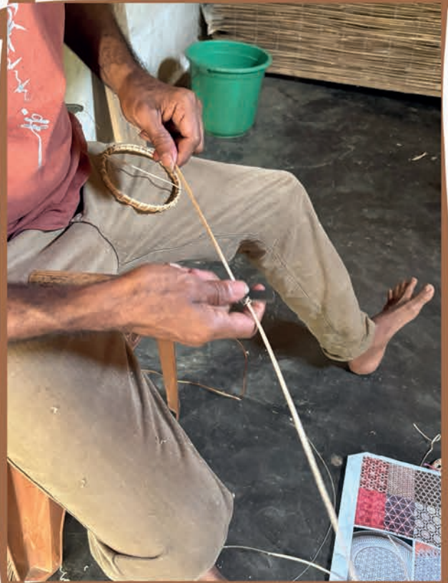
Scraping off the back of the strips to make it more flexible and light-weight
