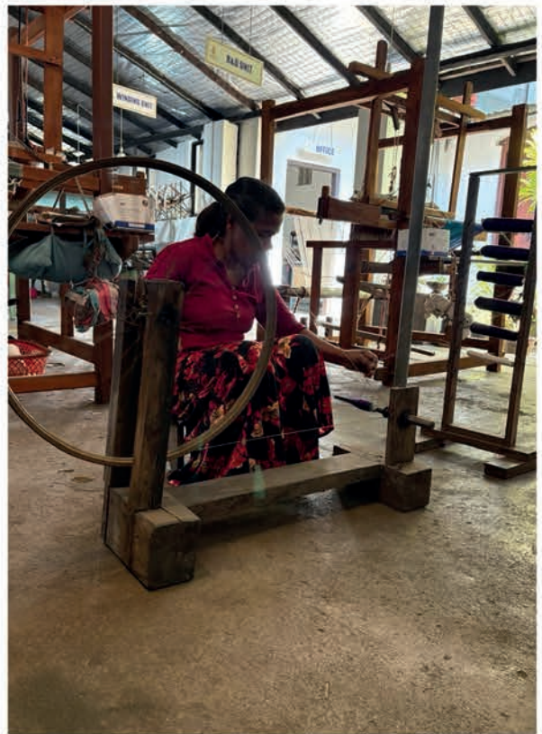
This is a weaving wheel, or more commonly a spinning wheel, is a traditional device used to twist fiber (cotton) into yarn for weaving.
