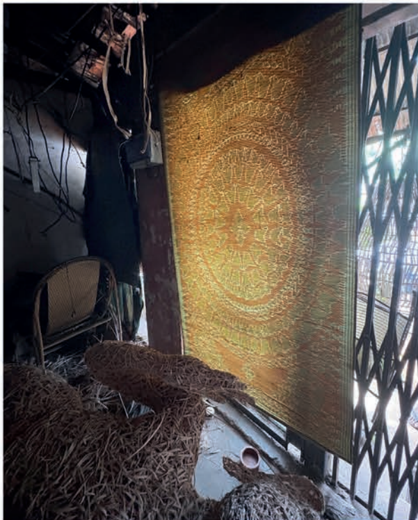
Workshop covered in pan mats to block the sunlight, because it could affect the quality of the materials
