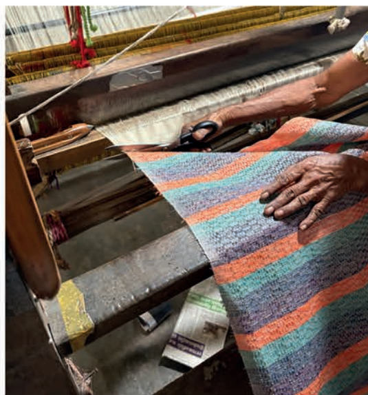
Cutting the fabric, they weave another inch from the edge before cutting to seal the weave
