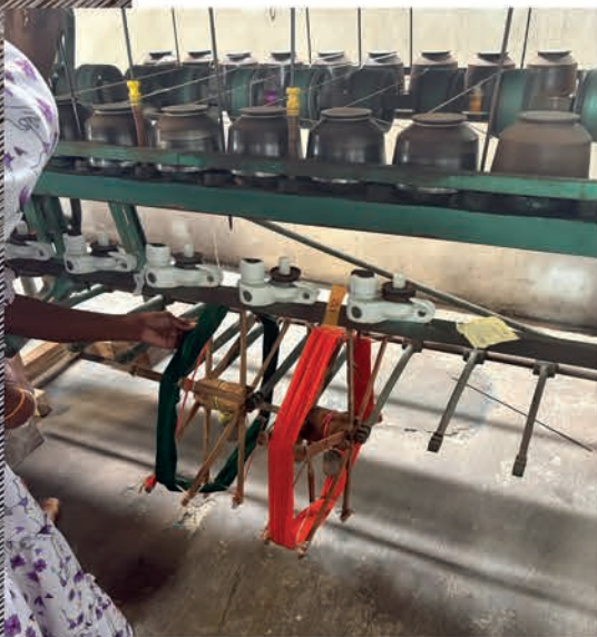
Winding the bobbin with the selected yarn
