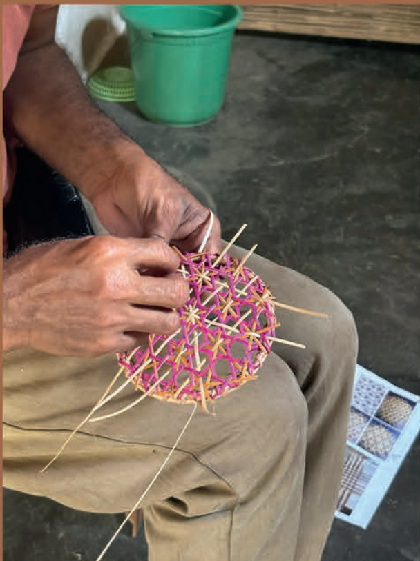
Weaving the samples in a round frame, because it's difficult do the weaving on a flat surface.
