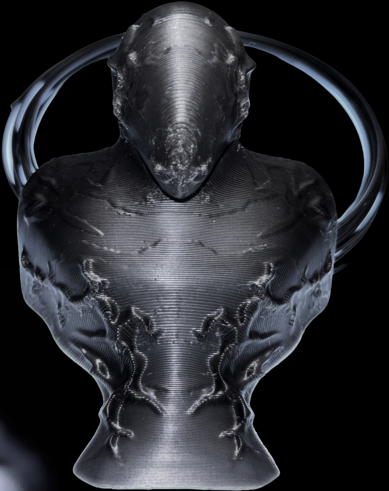
Capsule cover FDM printed with CHARBORN filament
