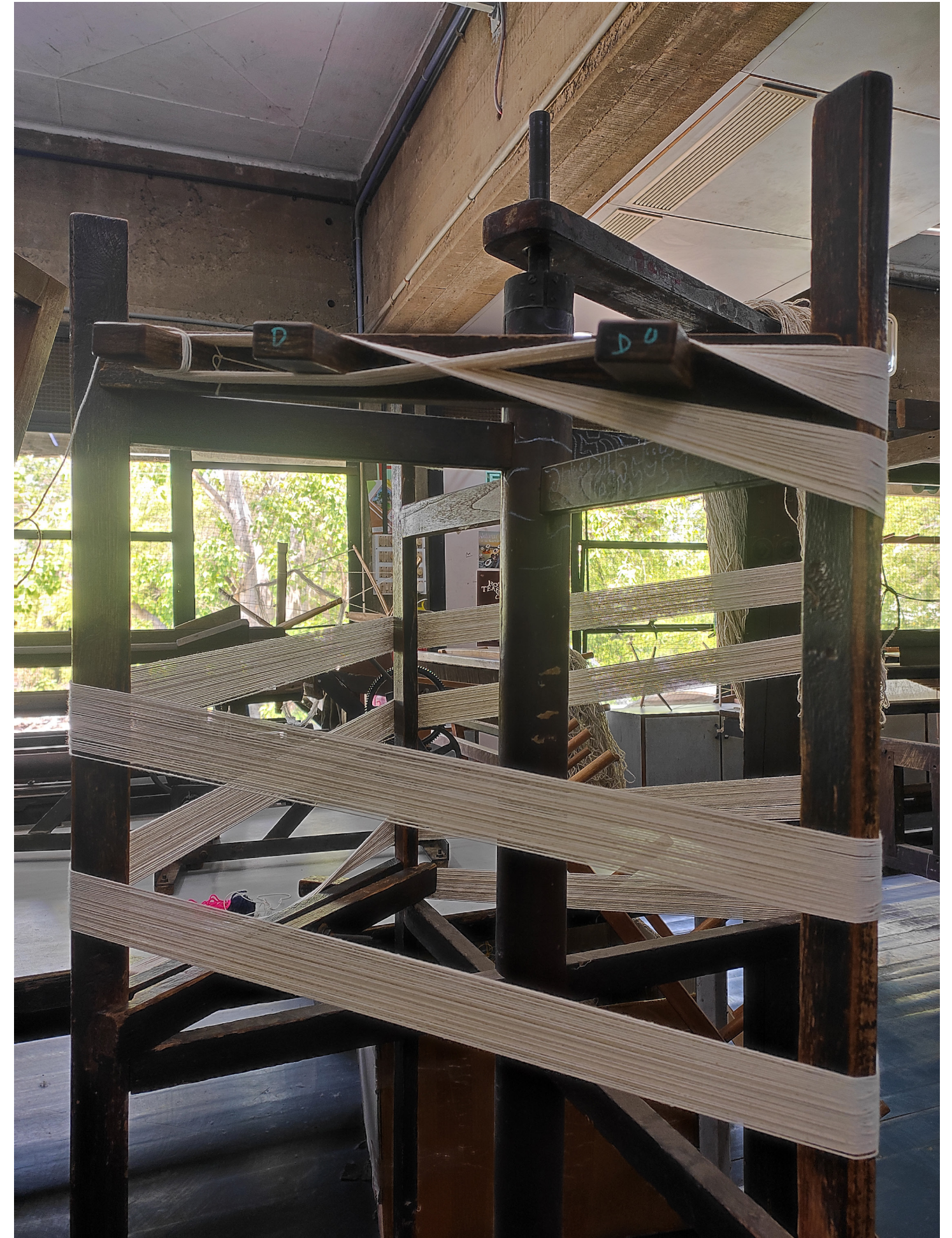
Warping in sections of 84 ends; thrice
