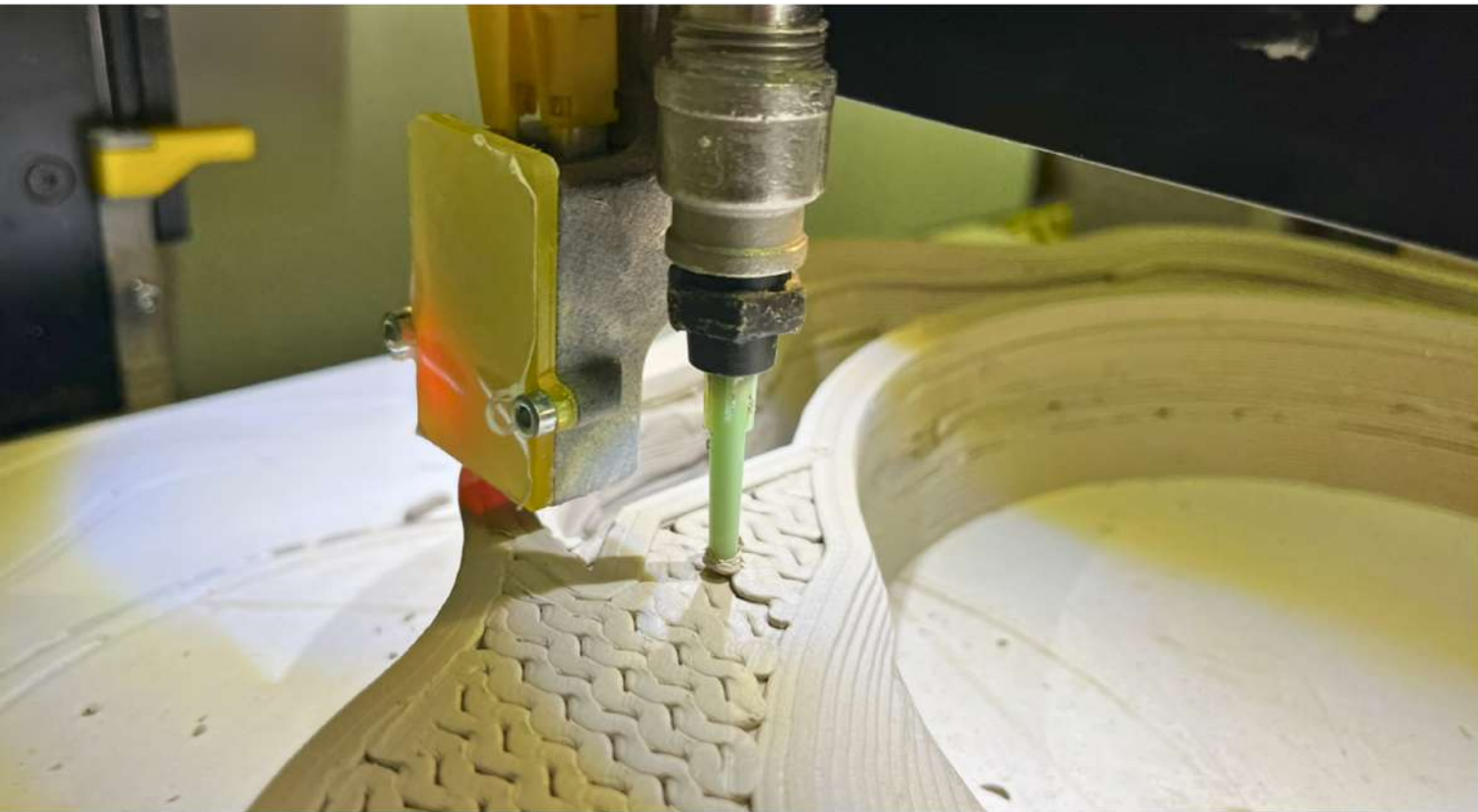
THE MODEL WAS PRINTED ON THE LUTUM 5 CERAMIC PRINTER.
