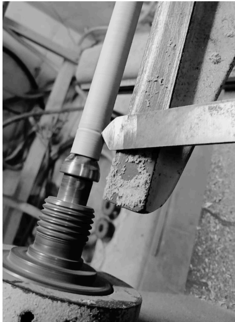
Making of wooden locking mechanism using Rosewood and magnets
