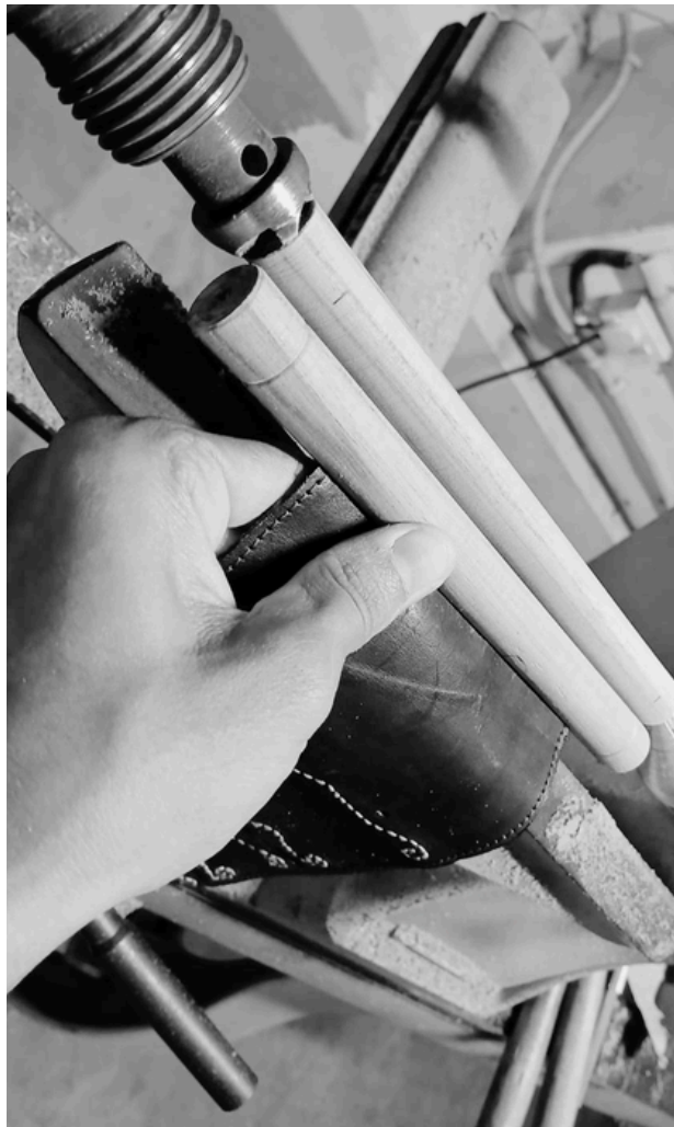
Making of wooden locking mechanism using Rosewood and magnets
