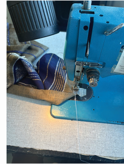
Gathering the skirt with a zig-zag stitch while keeping a strong thread inbetween the zig-zag to gather the skirt easily
