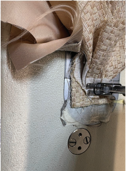
Attaching the front and back from the side seams and the inseams
