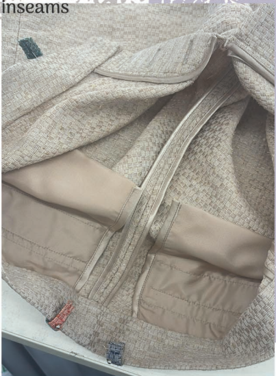
Attaching the waistband the beltloops: beltloops are attached to the waist first before attaching the waistband
