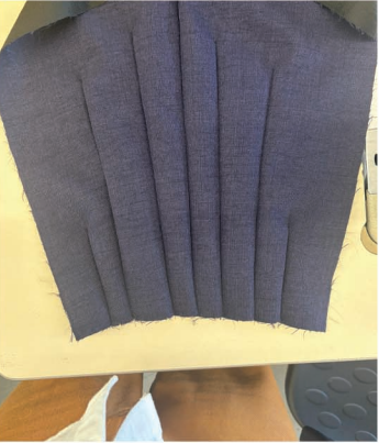
Doing the darts of the trousers from the bottom hem
