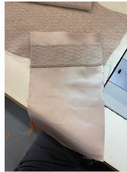
Attaching the pocket bag facings for the jet pocket
