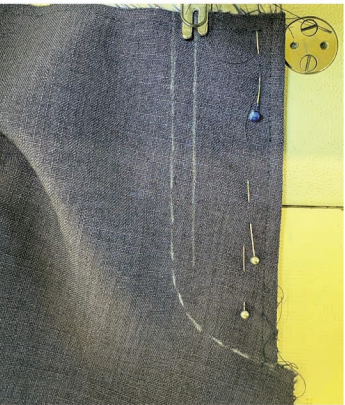
Top stitching the fly after doing the button holes
