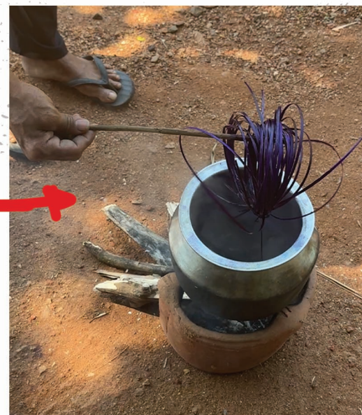
Boiling the cane in purple dye, it has to be boiled for about 20 minutes to get a dark shade
