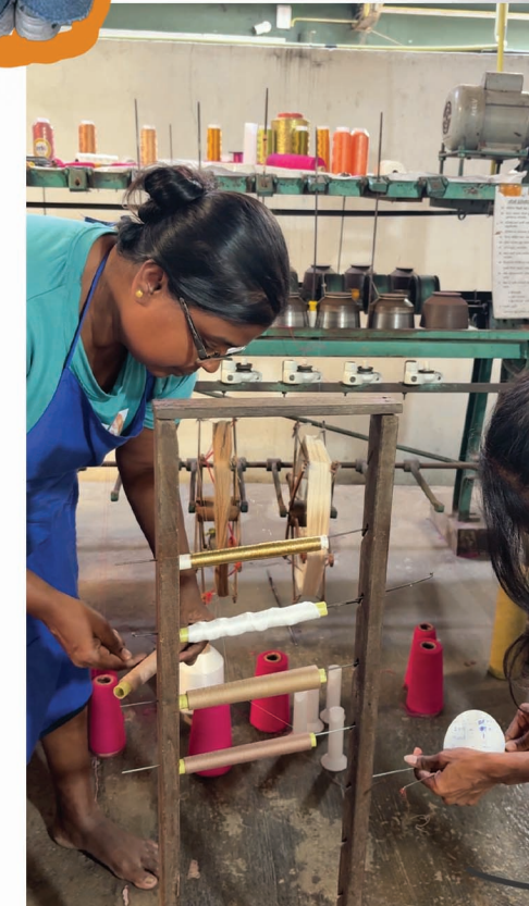
Bobbin winding for handlooms involves transferring weft yarn onto small bobbins using a hand-cranked or electric winder, ensuring it is packed tightly, evenly, and not overfilled to prevent snags in the shuttle. Key techniques include building up the ends first, maintaining consistent tension, and using a crisscross motion.
