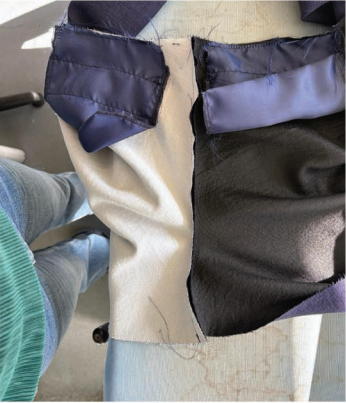
Doing the jet pockets from the back
