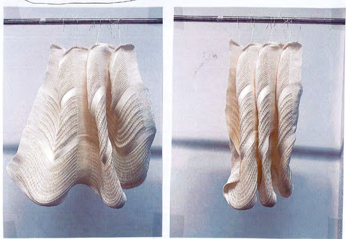
Sample of paper yarn controlling the movement of the textile
