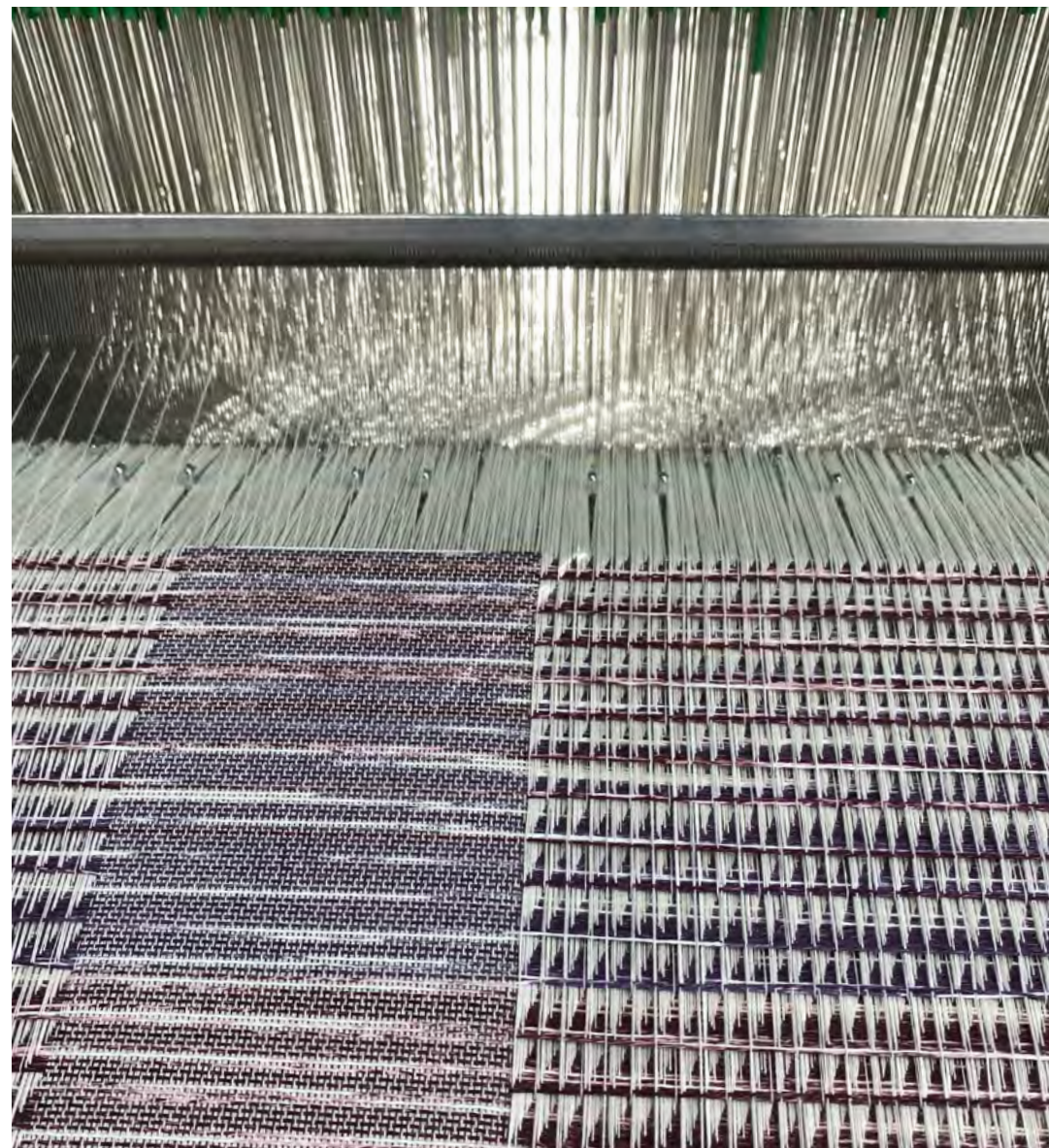
Process of weaving mist on jacquard loom
