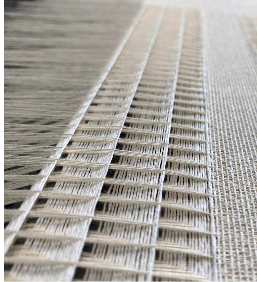
Process of weaving samples for Mist on jacquard loom
