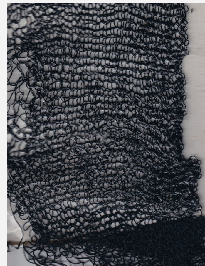
Knit + biofilm (Recycled yarn, probably silk and glyserol, pektin and carrageenan)
