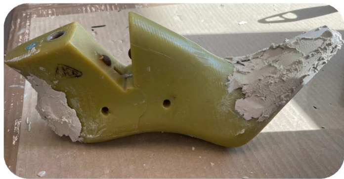
Modification of the shoe last using filler
