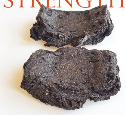
THE MATERIAL HAS A COMPRESSIVE STRENGTH OF 3.44 MPA WHEN ORANGE PEELS ARE REMOVED FROM THE RECIPE
