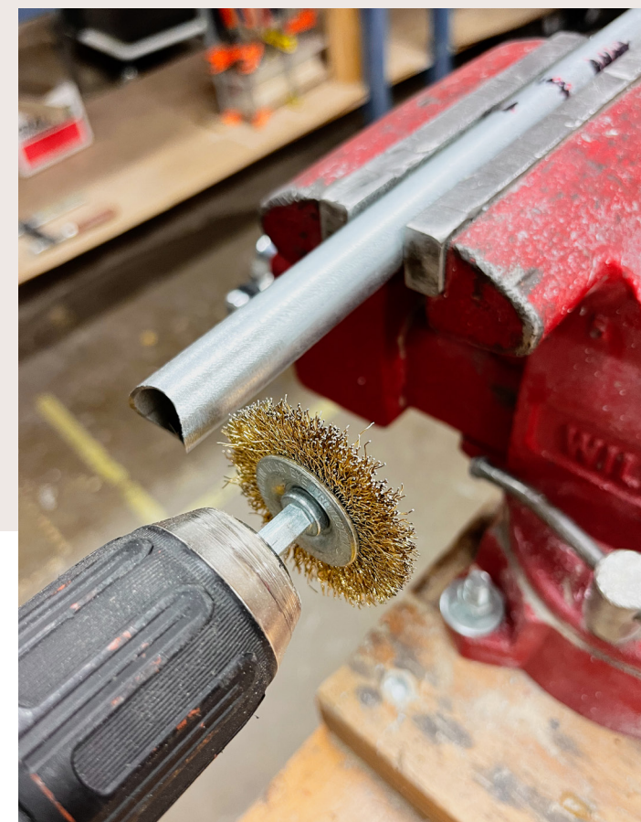
Sand Down the Joints
