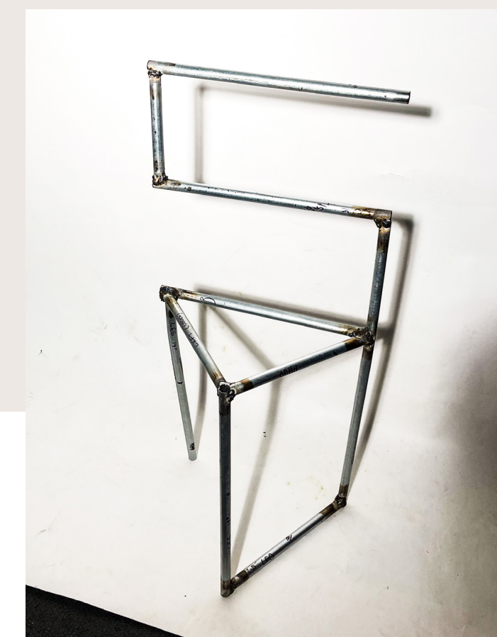
Weld the Pieces Together
