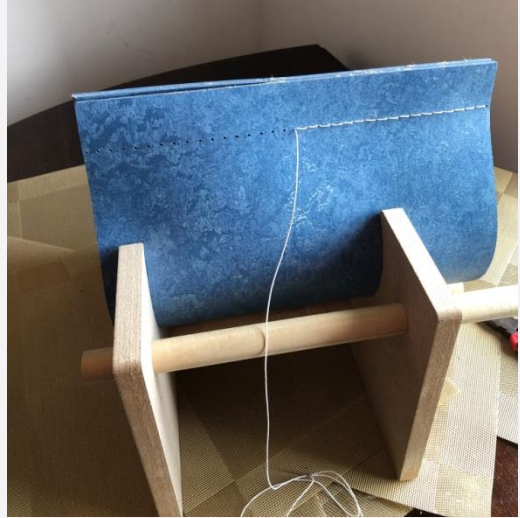
Utilising a jig to hold the two layers of linoleum in place when sewing them together.
