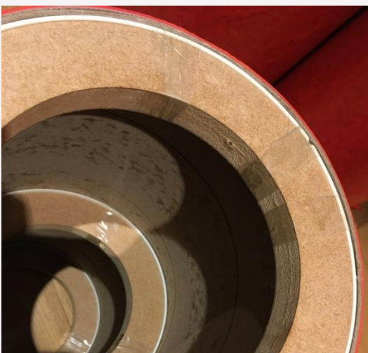
Three wooden rings inside the cardboard tube for structural support. Experimenting with a white detail around the edge
