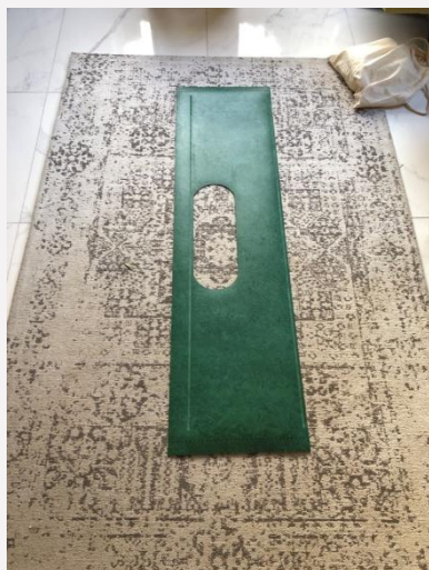
Cutting a curved slot into both layers of linoleum.
