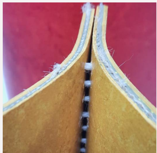
When sewing linoleum, the surface layer began to crack from the force applied to get the needle through
