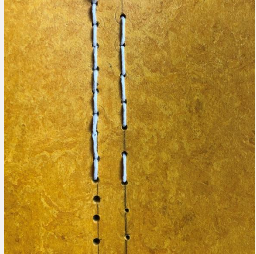
Experimenting with pre drilling holes to prevent cracking the surface layer of linoleum when sewing.
