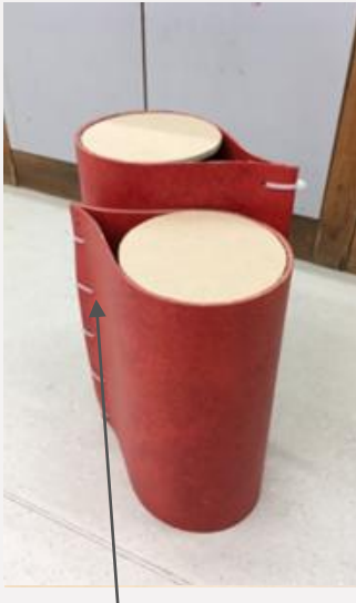
Linoleum fixed into position at the back
