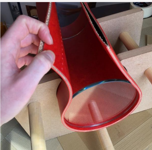
Further development of a jig to better hold the glass in place when sewing the layers of linoleum together.
