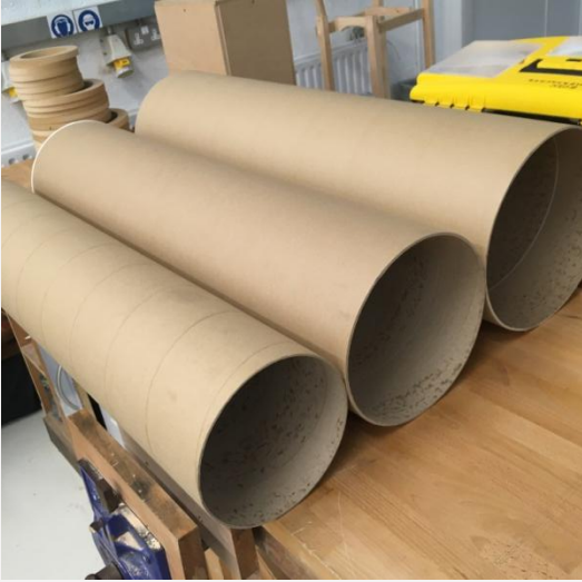
Cardboard tubes with diameters of 350mm, 300mm & 250mm. The largest readily available standard sizes
