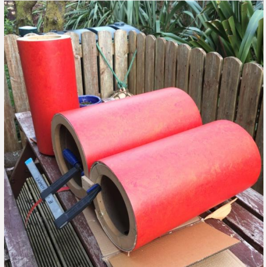
The cardboard tubes covered in lino
