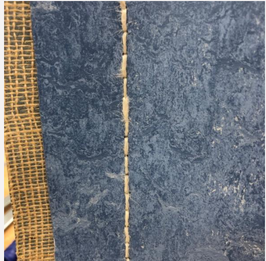
Cotton thread with a 12mm stitch length. The thread began to fray quite easily
