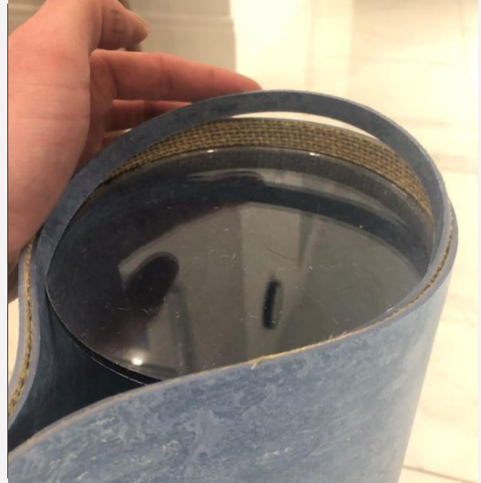
A cut is made through the internal layer of linoleum for the table top surface to sit on.
