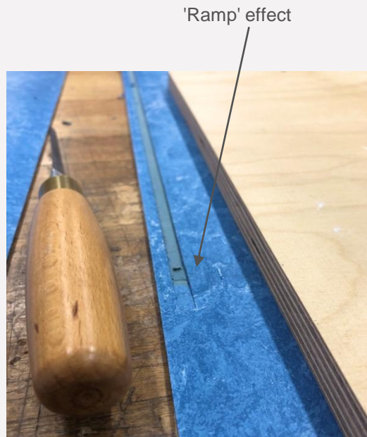
Cutting the rebates with a 3mm chisel. This took a lot of concentration to get right. Also I created a 'ramp' at the end of the rebate for the table top surface.
