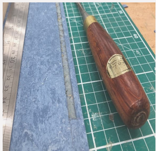
Cutting a 1.5mm rebate into the linoleum for the table top to sit in.
