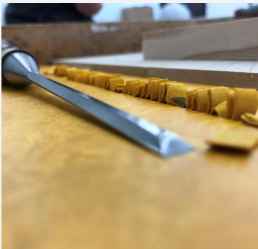
Cutting the rebate with a 6mm chisel.
