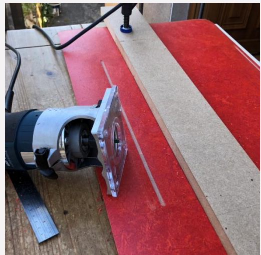
Cutting the rebate with a router.
