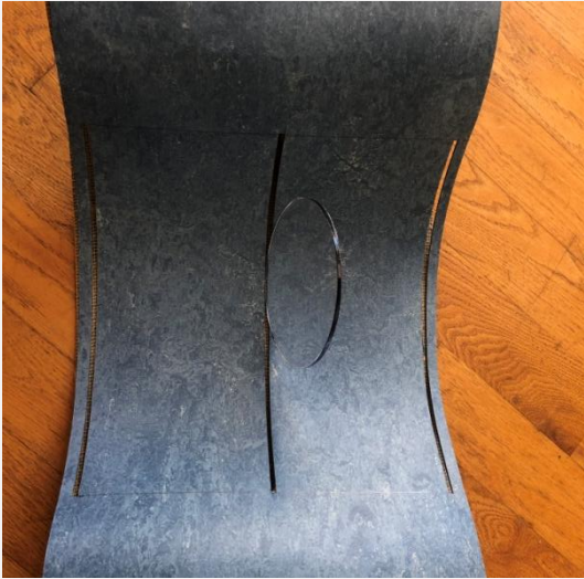
Experimenting with three rebates. Accidentally cut the rebates too deep.
