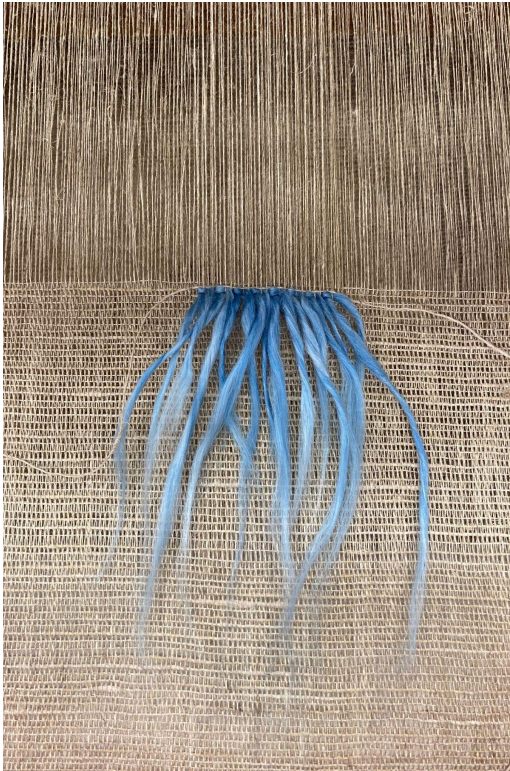
Ramie fibre, brushed spun by hand into small strands, dyed with Indigo
