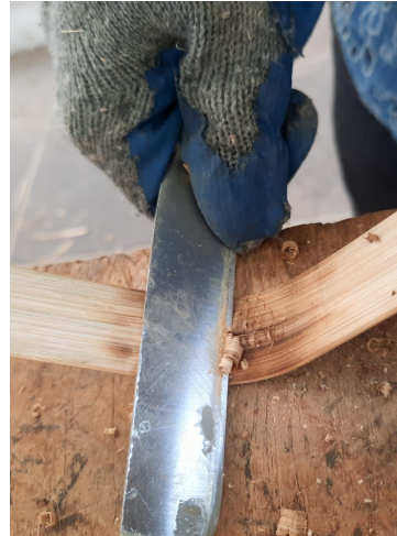
Heat Bending to expand the size of the smaller loops due to the shrinkage, and cleaning the burnt parts of the loops
