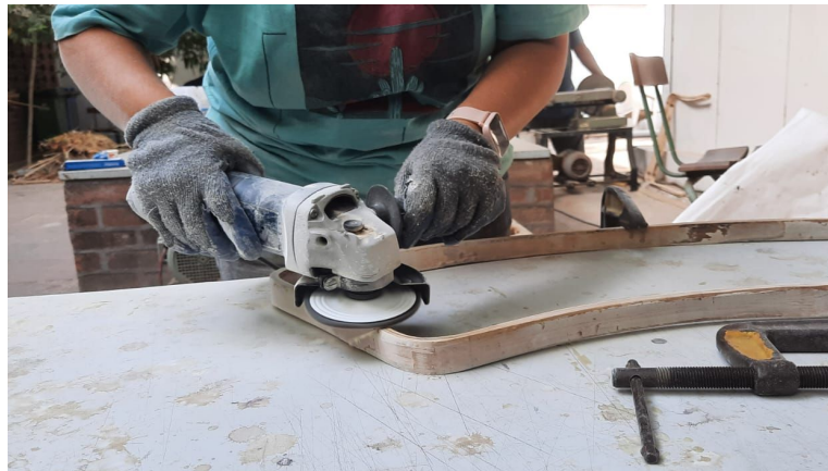
Finishing the Laminated loops, Removing Araldite, Making groove cuts for the lap joints, Sanding the skin off from the strips
