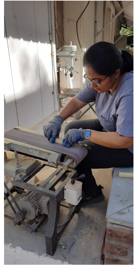
Shaping of the spine to fix the handle
