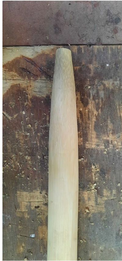
Shaping of the spine to fix the handle
