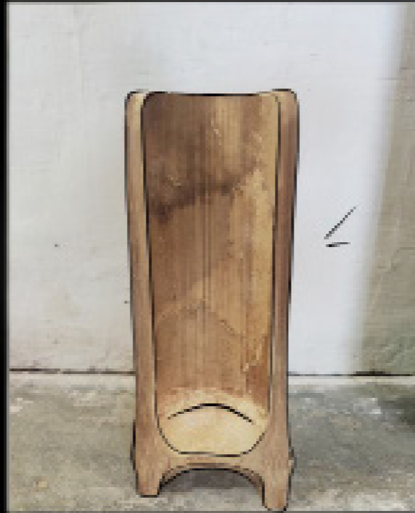
Splitting with an internode to get the base for candles to be held.
