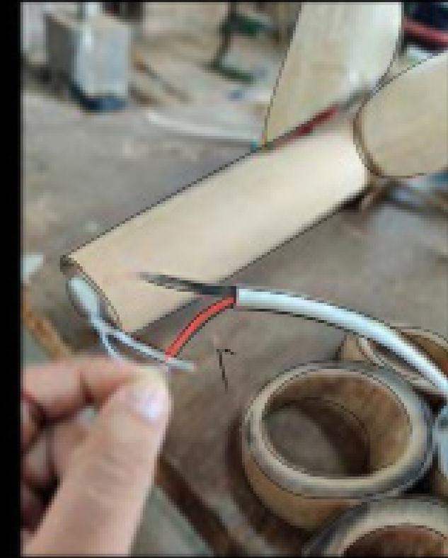
Wiring and fixing of light in the stem structure
