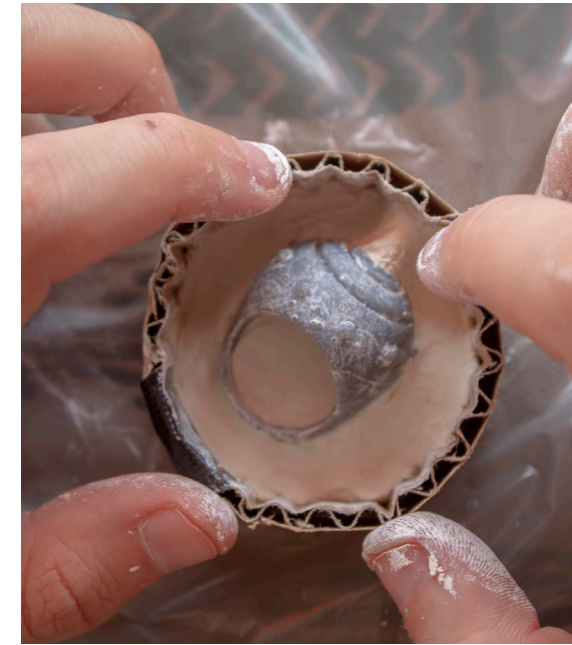
First steps for the prototyping of the silicone moulds: Put the ring inside the cardboard and fill half of it with moulding clay.
