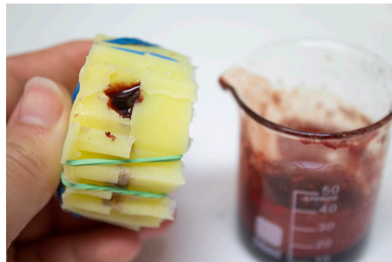
Filling of the ring mould by the material injection channel.
