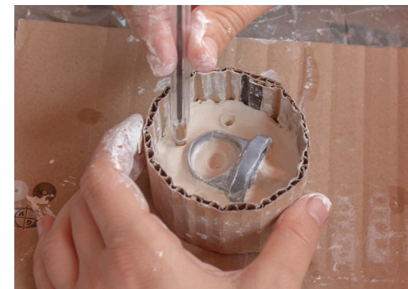
Create holes to generate lugs in the silicone mould.
