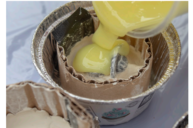
Pour the silicone to create the first half of the mould.
