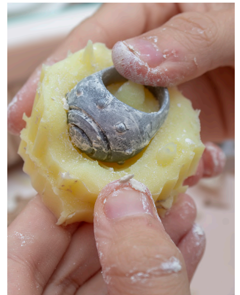
Demoulding of the 3D printed ring and obtaining the first half of the mould.
