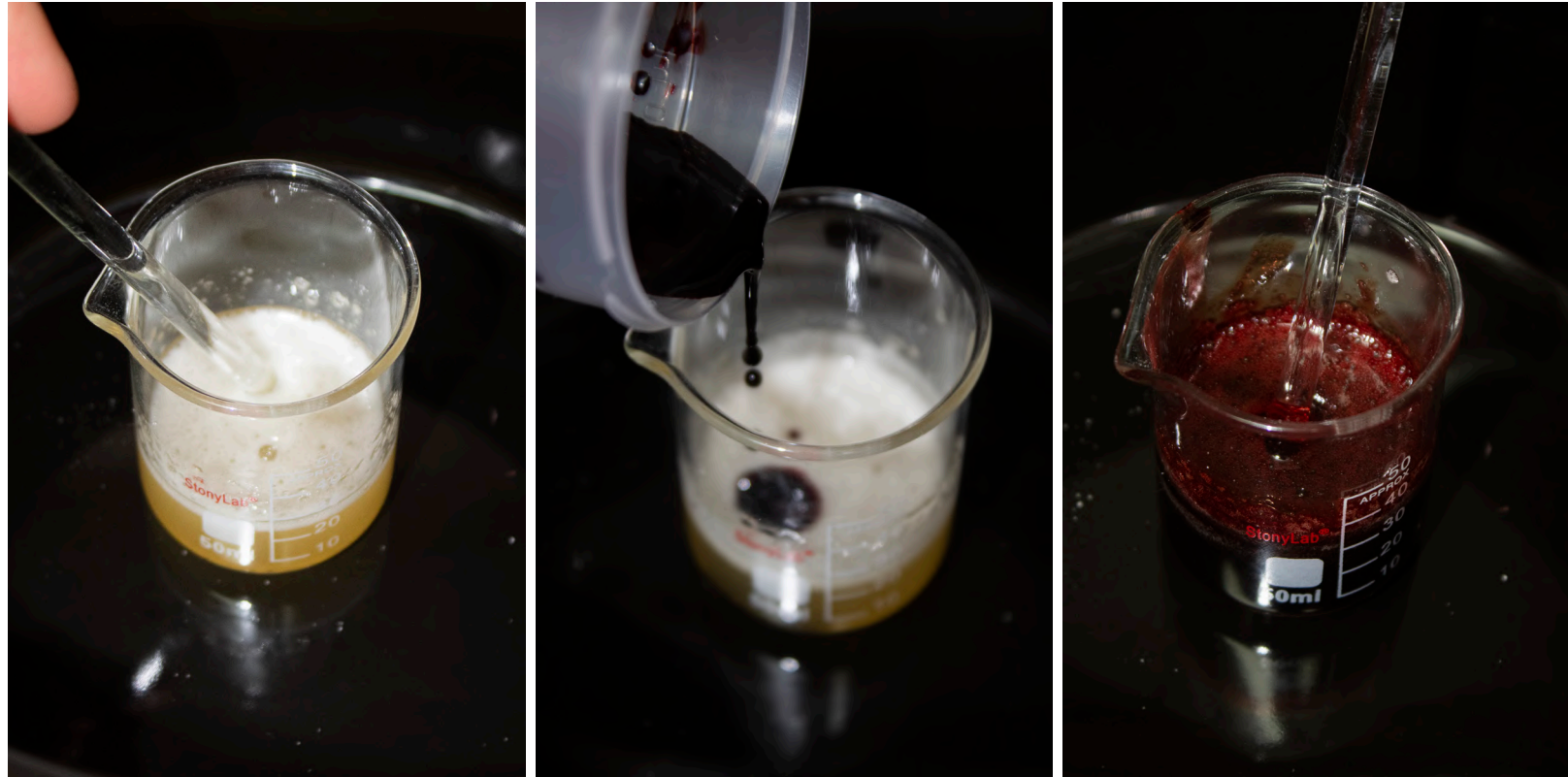
Prototyping of the new material (left picture, cooking of the gelatine with water/ middle picture pouring of the blood into the mixture/ right picture cooking of the complete mixture ready to be poured into the corresponding mould).
